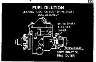
Another probable cause for dilution is in the injection pump. The pump drive shaft incorporates a double seal arrangement at the front of the pump. One seal is to prevent fuel (under approximately 10 PSI pump housing pressure) from entering the crankcase and the second seal contains engine oil in the crankcase. The two seals have a dead air space between them.
