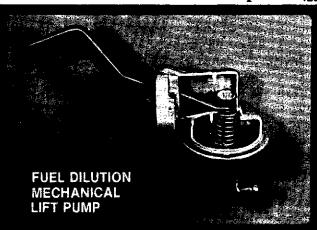
The mechanical lift pump is a single diaphragm pump and all fuel is contained below the diaphragm in the inlet and outlet circuitry of the pump. The inlet and outlet of fuel is controlled by two check valves contained within the pump. The pump also contains a shaft seal.
