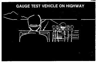
Operating vehicle on highway with gauge bar instrumentation in cab would primarily be used when a stalling or severe loss of power is experienced when operating the vehicle at highway speeds and inshop diagnostics do not indicate a problem.
