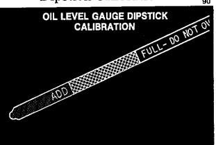
Correct oil level gauge calibration can be verified by draining the engine oil and filling the engine/oil pan with nine (9) quarts (8.5 liters) of oil. Assuming that the oil level gauge is properly seated, correct oil level gauge calibration is indicated if the oil level is within 1/16 inch of the "full" mark.
