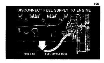
4. Remove chassis fuel supply hose to mechanical lift pump at the steel fuel line just downstream of the mechanical lift pump. Installing a Vice Grip on the hose prior to removal prevents filter draining.
