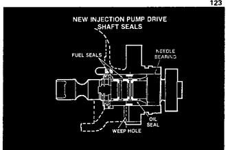
A three seal design (two fuel and one oil) and an external weep hole between the oil and fuel seals has been incorporated into the 6.9L injection pump beginning with the following engine serial numbers:
