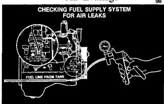
To determine if suction side leak exists, remove supply line (hose) from mechanical lift pump and apply 3" vacuum to the removed hose and vacuum decay should not occur. If vacuum does not hold, a suction side air leak exists and repair is required.
